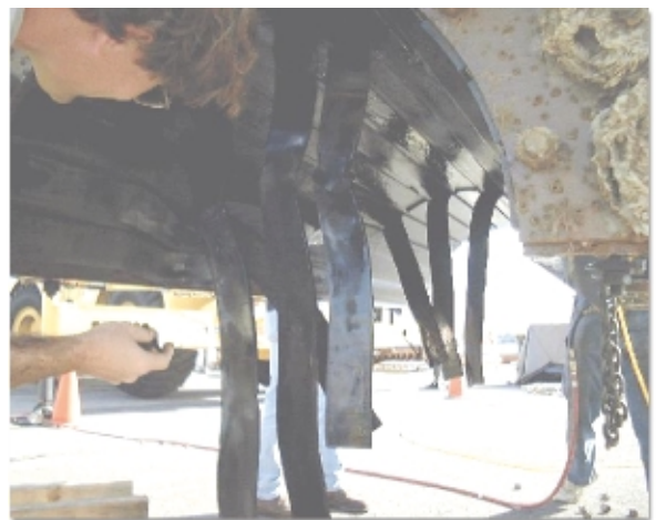
Geoff Healy inspects the damaged bearing staves.
